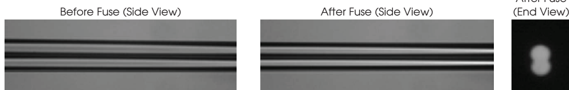
View from the glass processor of two single mode fibers tapered and fused together for 50:50 coupling. Spacing between the fiber cores is approximately 15 to 20 µm.
