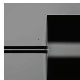
Ø1.25 mm Silica End Cap Fused onto Ø125 µm Fiber
