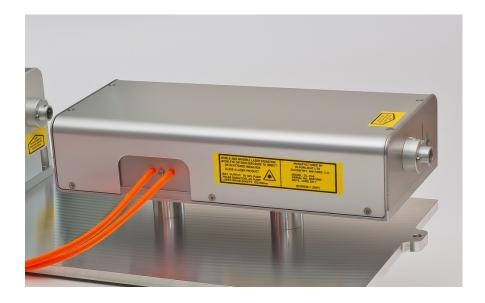
DL series dye lasers convert the output of Elforlight pulse lasers to other useful wavelengths, whilst maintaining the benefits of short pulses and high repetition rates. The self-contained dye reservoir and pump enable operation for several weeks on one dye fill. Options of broad and narrow (15 to <1nm) wavelength bandwidth are available.
